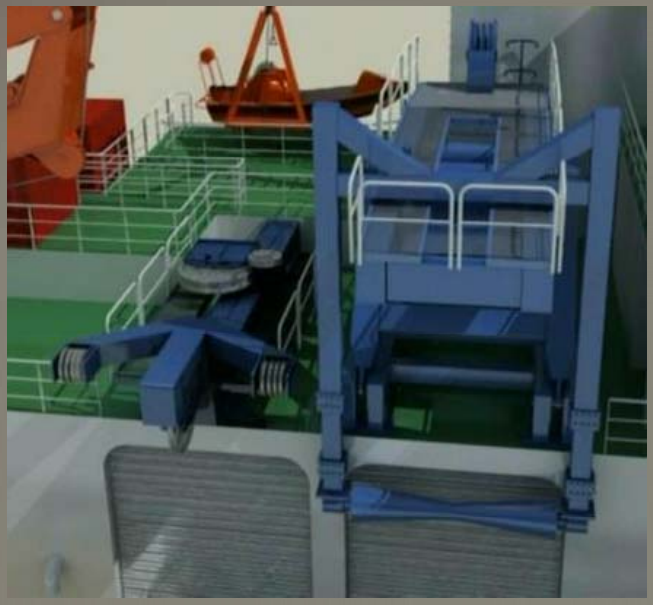
Starboard 'A' Frame Capacity – 20t Max. Height – 5m
